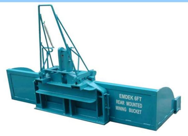
The EMDEK Tractor 3 point linkage mounted rear bucket is suitable for tractors of 45Hp and above. Models are available in various sizes with cutting widths of 6 feet and 7 feet. Working in reverse, the bucket may be tipped to unload earth. The machine is constructed of steel, a grader blade cutting edge is welded. Ideal for leveling land, Cleaning harvester's paths, moving earth, building bunds both in plantations or construction sites.
