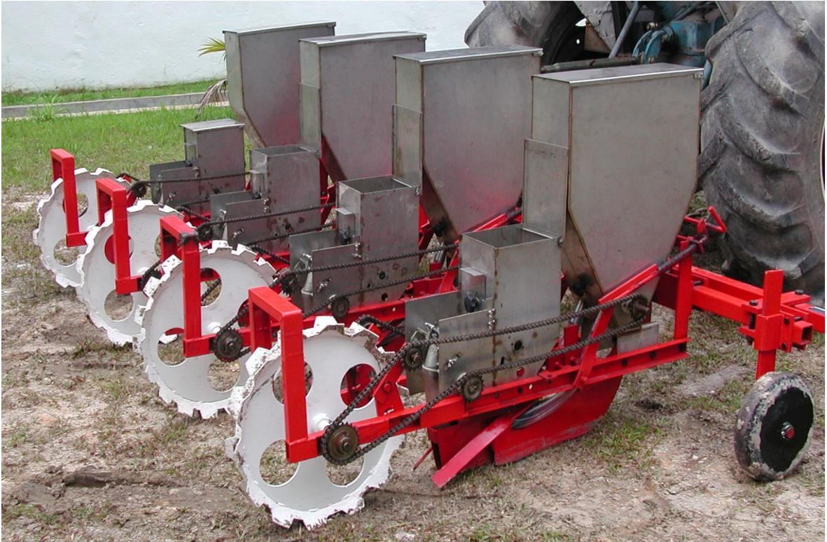
Suitable for Corn, Peanuts and other similar size seeds. Rotary plate operation driven by press wheel through sprockets and chains. Seed and granular fertilizer boxes constructed of stainless steel, plates of aluminum supplied drilled according to customer planting requirements. A selection of seed plates are available for different seed sizes and thickness. Rear press wheels of steel. Twin toolbar with three point linkage headstock.
