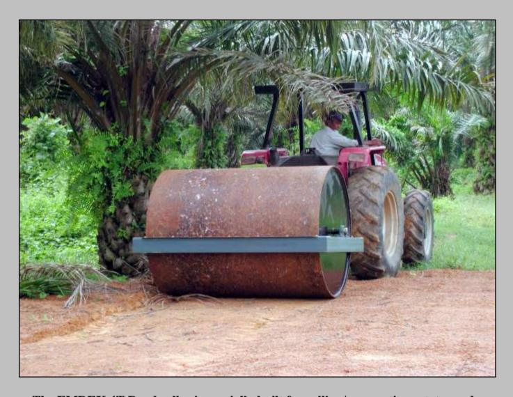
The EMDEK 4T Road roller is specially built for rolling/compacting estate roads. When empty, it is 1.5 tonnes in weight to allow for easy transportation from estate to estate. And when filled with water, the gross weight is 4.2 tonnes giving excellent compaction ability. The machine is constructed from heavy gauge steel and heavy duty bearings. Drum has 2 screw-on plugs to allow for draining and filling. Suitable for use behind a tractor with minimum of 70 HP prefereably with 4WD.
