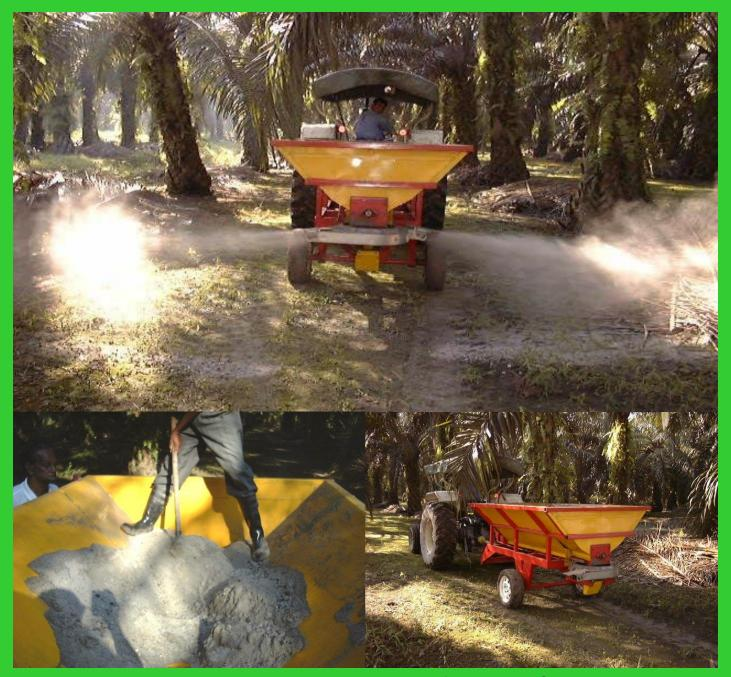
The EMDEK Bunch Ash spreader has a welded steel frame with M.S. hopper to carry approximately 1.5 tons of bunch ash, single 3 ton axle, auger feed with chain reduction gearbox, 750x16 rims and retread tyres, stainless steel spreading mechanism with grease lubricated gearbox and deflectors, 2 PTO drive shafts, flow control with lever. 6 stainless steel spreading vanes. Wire mesh screen and PTO shaft included.
