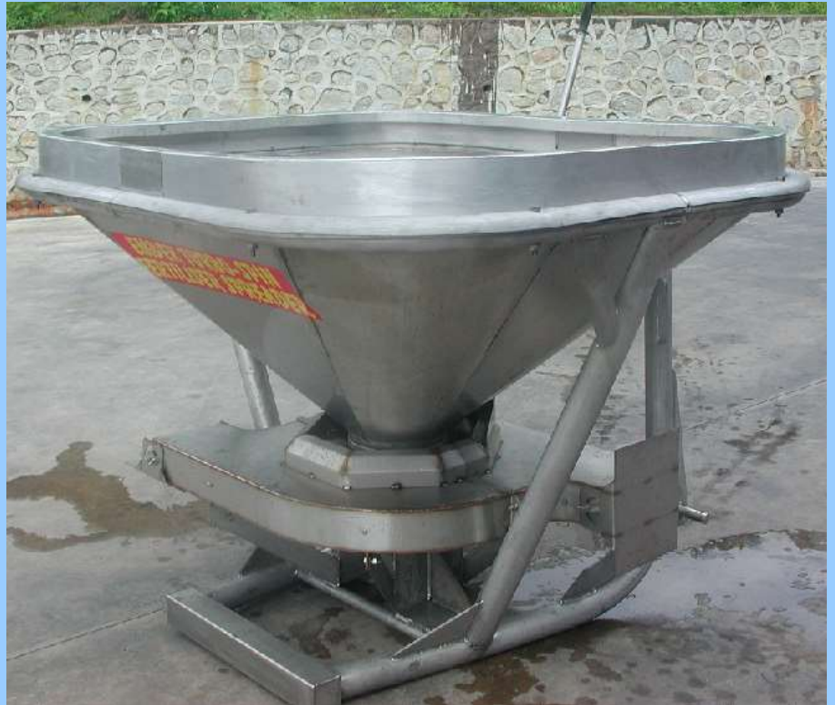
Stainless steel frame and spreading mechanism
