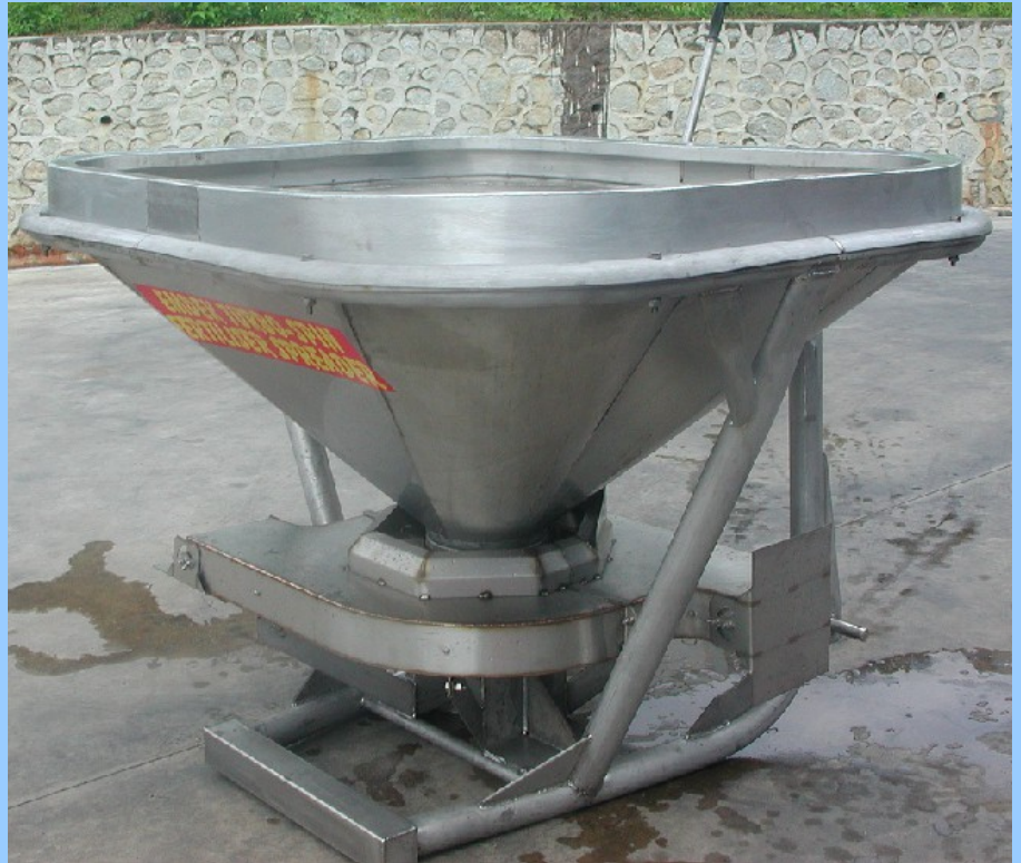
Stainless steel frame and spreading mechanism
