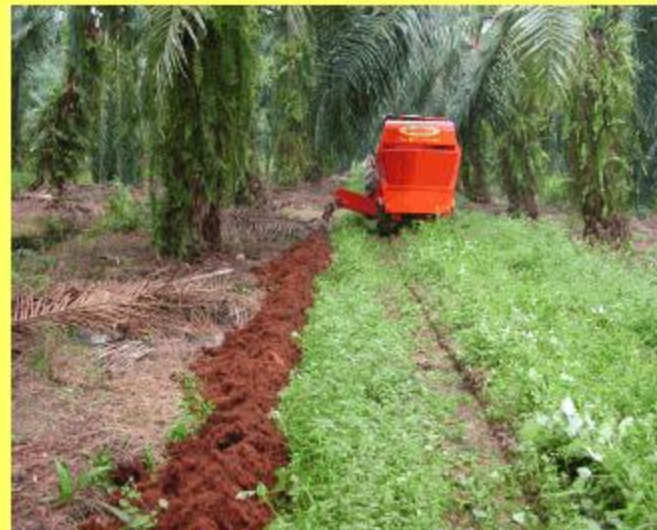
Resultant chopped material discharged onto side of machine into palm path of 10-12 tons per hectare
