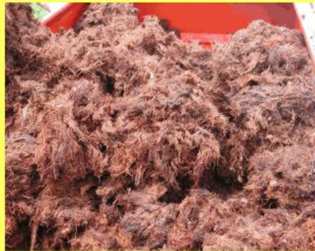
Empty Fruit Bunches placed into the bin and chopped for 10 mins.
