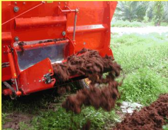
Hydraulically driven and controlled discharge chain conveyor
